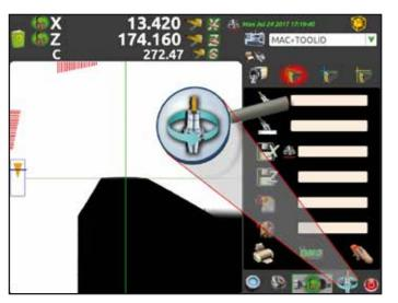
Autofocus function: all new operating mode and capability that allows the machine to measure automatically the tools, without operator presence.
