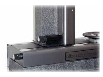
Micrometric registration of X and Z axes by means of two wheels which are essential for the collimation of the measure with a fixed target function.
