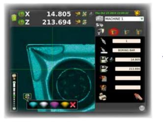
Inspection function for accurate control of the tool status. Possibility to increase or decrease the brightness for a better visibility.
