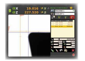
Td SIX is a new software function developed by Elbo Controlli, used to acquire tool's measurements, to input them into the tooling tables and create a file including tools offstes.
