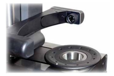
Camera system for measuring with punctiform illuminator and inspection with ring illuminator.
