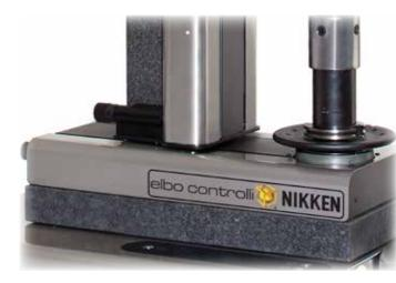
Base and column made of ground granite. The thermal inertia of this material allows the machine to be placed directly in the workshop. Mechanical elements manufactured from stainless steel.
