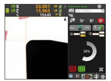
Software displays the measuring progression during the automatic acquisition cycle of the cutting edge by circular percentage loader.
