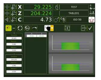
**Autofocus** function: automatic search and measurement for single edged tools.
