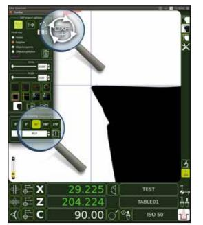
DXF profile creation fuction: automatic rotation of the tool to memorize the geometry developed and built up during full spindle rotatation to automatically generate a DXF drawing.
