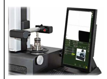
The presetter E46L is equipped with a 22" capacitive touch-screen monitor, mounted vertically for easy viewing. The screen layout and design is split into two distinct sections. The upper half of the display shows visible images of the current tool and profile. The lower half shows and allows access to all the current software functions. The operation is very intuitive and logical to allow the operator to interact with the machine and software without having to attend complex trainings sessions.
