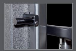
Manual axes movement. Axis unclamping by means of a single pneumatic control system. X and Z axes block management with control maximum speed of translation 2mm/sec.
