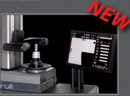
Large 15" touch screen for the best visualization of the tools and simple management functions to operate the measuring machine.
