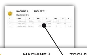
It's possible to generate and / or print a report with the theoretical values, tolerances and measurements of the selected tool table.
