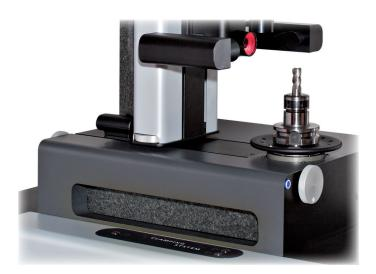
The base and the column, made of ground granite, are increased substantially in size over the previous generation model to guarantee and maintain maximum accuracy. The low coefficient of thermal expansion from this natural material allows the location of the machine directly in the workshop with no issue or concern in respect of accuracy and performance.
