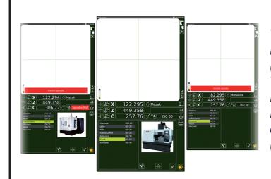
The new software also includes automatic recognition of the spindle via SP-ID (Spindle Identification System). This system allows the presetter to identify each spindle cartridge as it is loaded and suggest the correct machine origins, whenever the spindle is changed. (Optional)
