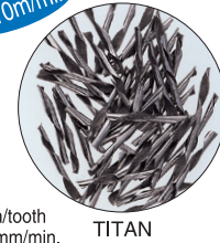
NC5-63 Material: TITAN V=75m/min. f=0.18mm/tooth S=1500min -1 F=1700mm/min.
