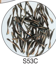
NC5-63 Material: S53C V=500m/min. f=0.25mm/tooth S=10000min -1 F=10000mm/min.
