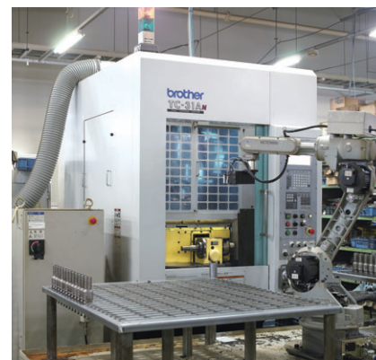
CNC table on TC-31A(pallet changer)+ work change by robot
